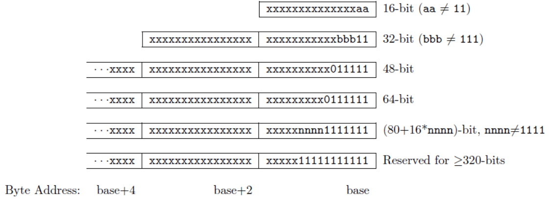
Figure 5: RISC-V instruction length encoding [2]
